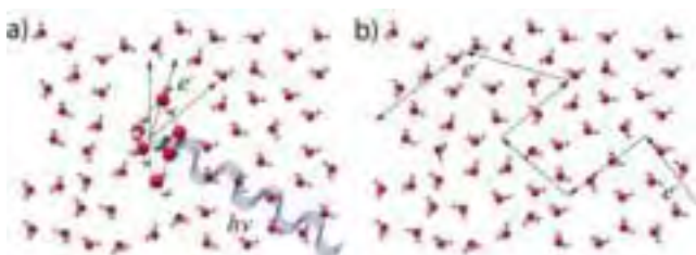
Figure 1: Electron scattering is assumed to be determined by the “local” scattering contributions (a) and the “transport” scattering contributions (b).
