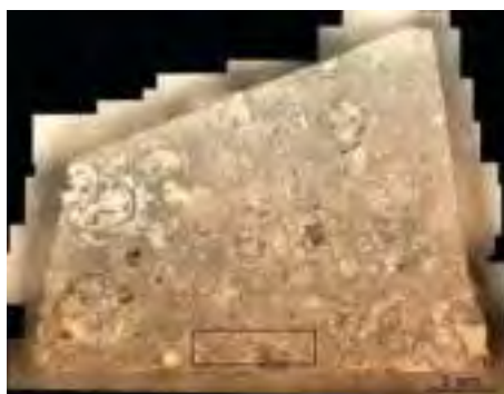
Fig. 2. Composite microscope image of an Allende meteorite sample. The surface area surrounded by the black rectangle was investigated spot-wise in detail by LMS using the femtosecond laser system (see Fig. 3).
